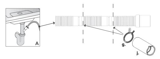
If the connection diameter is different than standard discharge hose connections, please use the connector piece provided with the machine with instructions illustrated.
