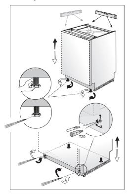
Adjust the front foot level by hand or slotted screwdriver to balance and raise the dishwasher to the enclosure height. Adjust the rear foot level with a screwdriver to balance and raise the dishwasher to the enclosure height.
