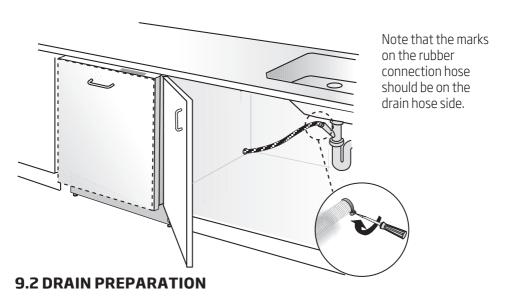
The dishwasher drain hose may be connected to the drain plumbing in one of three ways (Figure **A**, **B**, **C**).
