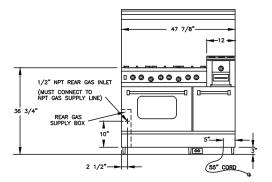
ELECTRICAL CORD LOCATED IN BACK OF UNIT LOCATION OF ELECTRICAL, OUTLET MUST NOT BE HIGHER THAN 3" FROM FLOOR IF LOCATED BEHIND THE UNIT OR CAN BE LOCATED IN AN ADJOINING CABINET.
